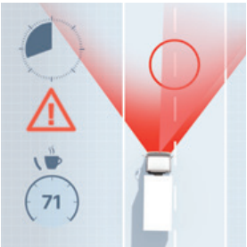
Attention Assist System When the truck is moving at speeds above 60 km/hr, AAS will alert the driver if the system detects any inconsistent steering input and will suggest that the driver takes a break.
