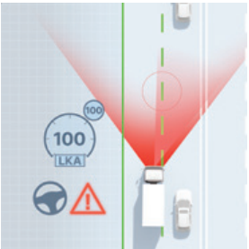
Lane Keeping Assist LKA works hand in hand with the truck's cruise control system, helping the driver to maintain lane position while in cruise control. This feature is able to steer the truck back into a central lane position if required. Only available on FV F Series 6-Cylinder models.
