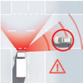
Intersection Warning System At an intersection, side-mounted short-range radars can detect obstacles or obstructions in the vehicle's path, including cars, bicycles and pedestrians, and alert the driver.
