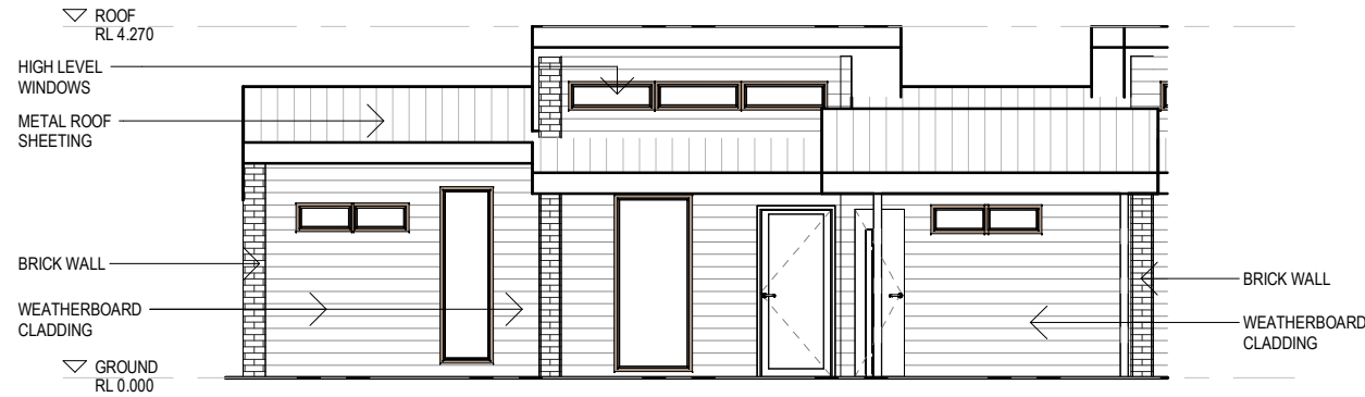
2 190 TYPICAL 2 BED UNIT NORTH ELEVATION 1 : 100
